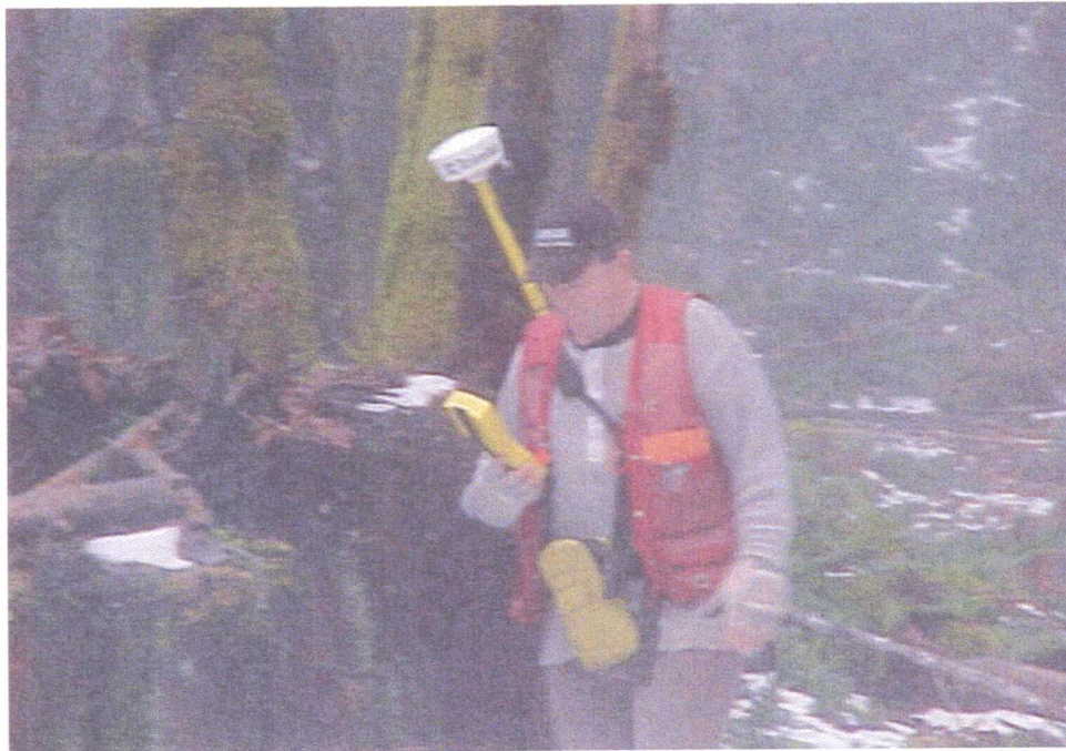
Fig. 24. GPS survey conducted in January 2003 using back-mounted differential GPS unit.
