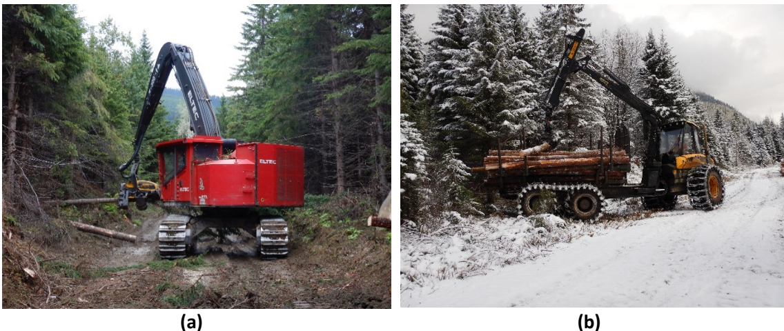
Figure 3. Machines used in CT operations: (a) harvester; (b) forwarder.
