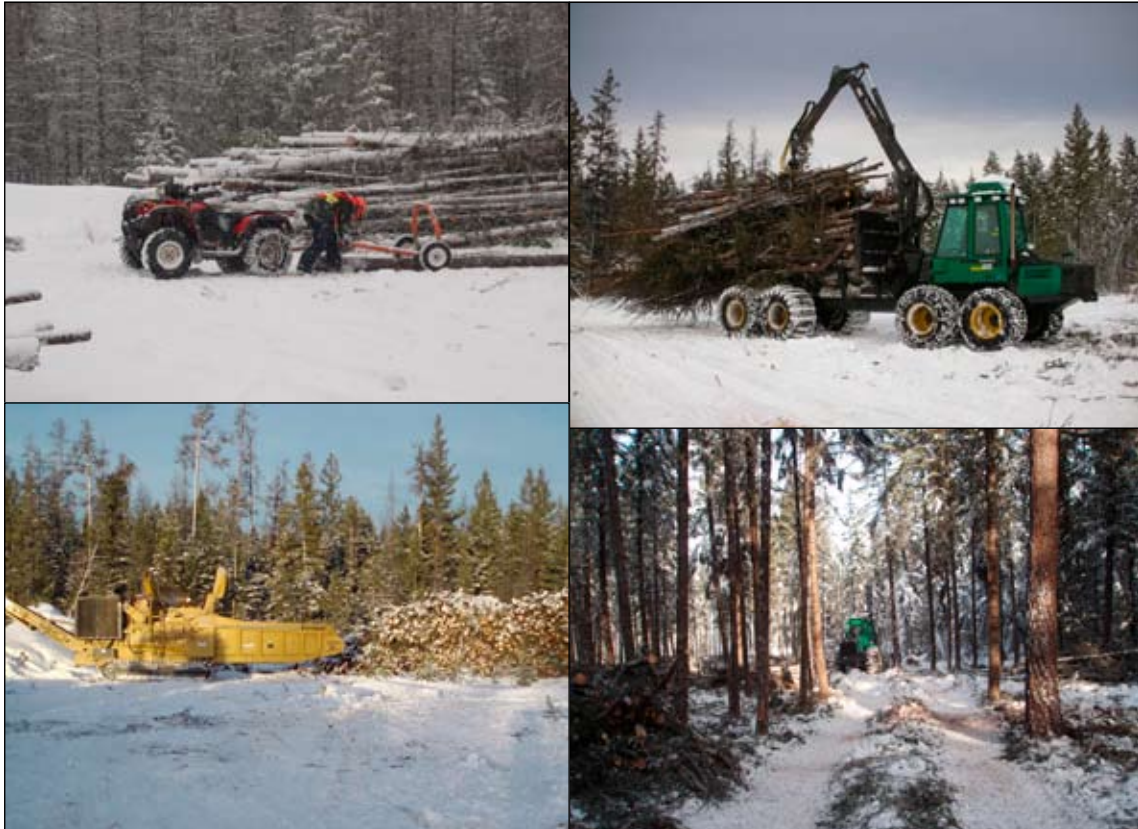
Figure 13: Williams Lake Municipal Airport fuel reduction in 2009, when 9.4 ha were treated. Clockwise from top left: Rolf Scheutze unhooks a turn from ATV with skidding arch; Nilsson Select Contracting with a forwarder-load of debris for stacking at landing; Nilsson Select Contracting harvester falling dead pine and damaged understory Douglas-fir; Pat Huska's grinder starting work on piled debris.
