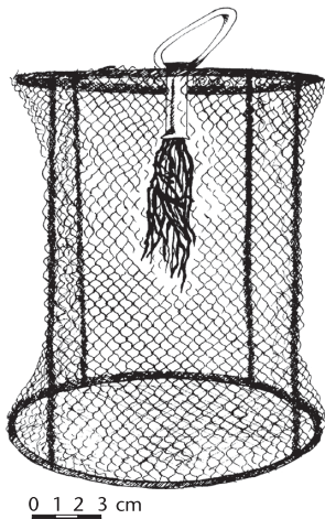
FIGURE 29 Mesh enclosure used for study of lichen growth rates.
