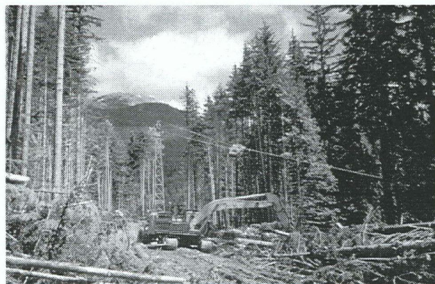
Figure 5. Loader clearing the landing during yarding.
