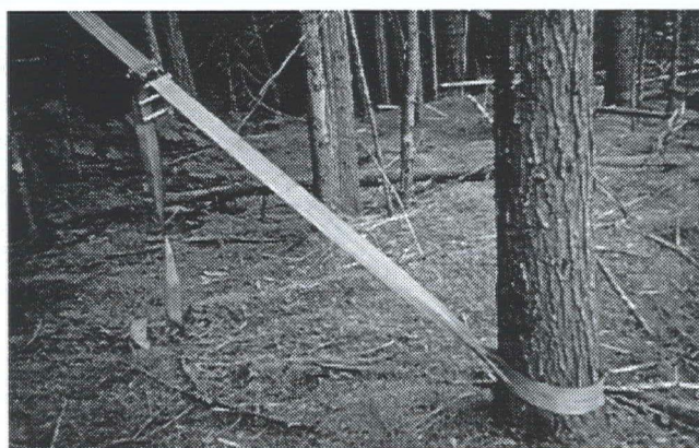
Figure 7. Nylon guyline strap with self-tensioning clamp.
