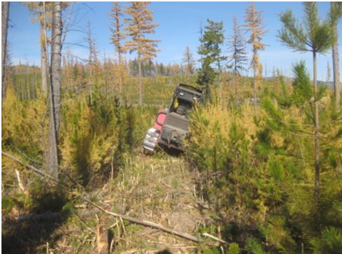
Figure 2. The mulcher tilting as it encountered a large stump.
